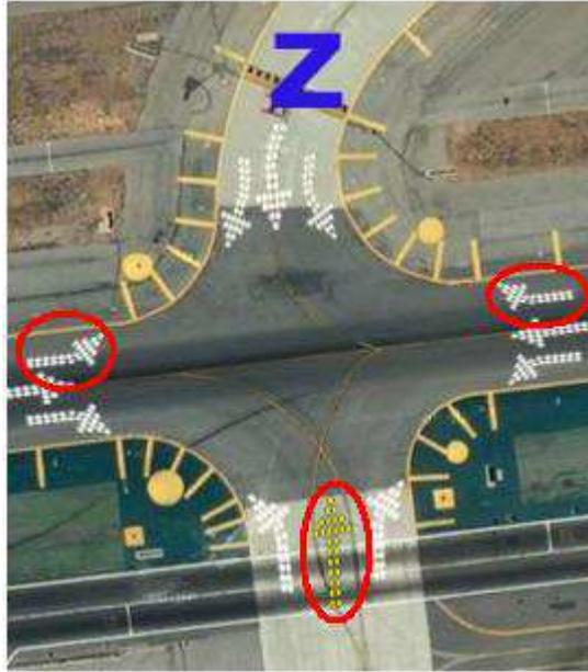
Taxiway Z has references to the circled arrow lights and is responsible for determining which one is lit when drawing a route.
