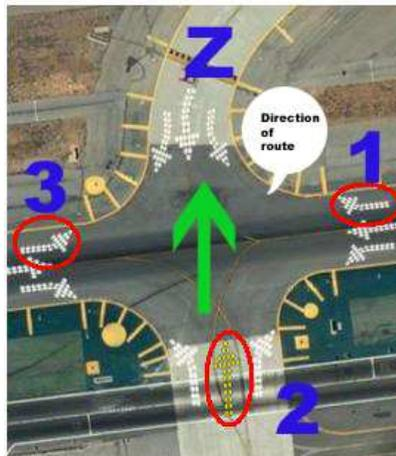
The current taxiway is Z and the previous taxiway is 2 therefore the middle light's state is set to ON and turned on when the route is confirmed.
