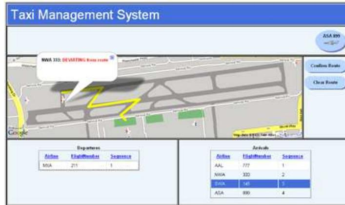
Display shows message box stating that the plane is deviating from its assigned route
