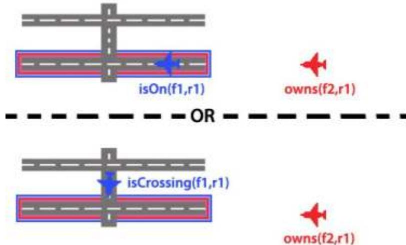
Returning to our example, the arriving plane has received the crossRunway message with the value “Two Four Left.” This fires the “isOn” rule for this airplane. The departing plane has received the clearedForTakeoff message with the runway “Two Four Left.” and the “owns” rule fires. Once this assertion is added to the knowledge base, the “incursingOn” rule fires and both airplanes receive the predicate “incursingOn” with the object “Two Four Left” in the knowledge base.
