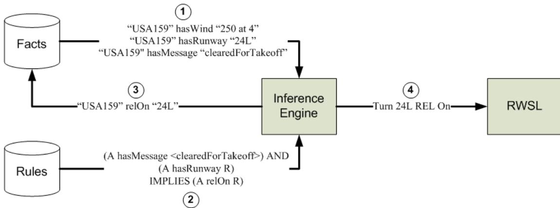
The rule states that if there is an airplane that has received a “clearedForTakeoff” message and this same plane is associated with a runway, then the RWSL system should be turned on for the given runway. Due to the existence of the hasMessage and hasRunway assertions about flight “US Air one five nine,” a new statement regarding REL illumination is added to the knowledge base.
