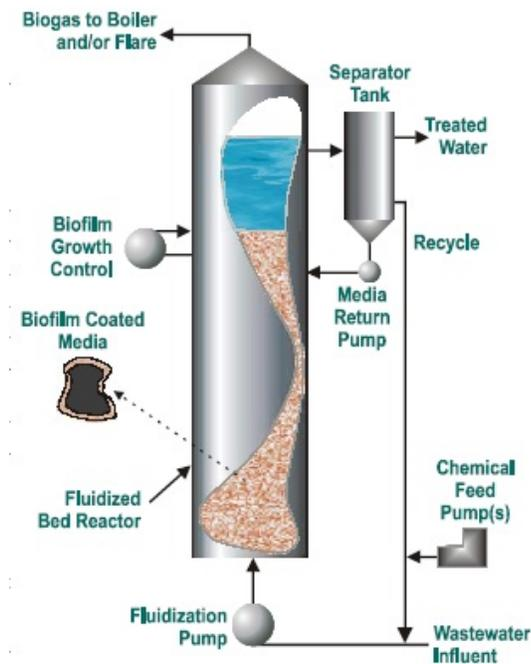
Figure 6. Anaerobic Fluidized Bed Reactor
