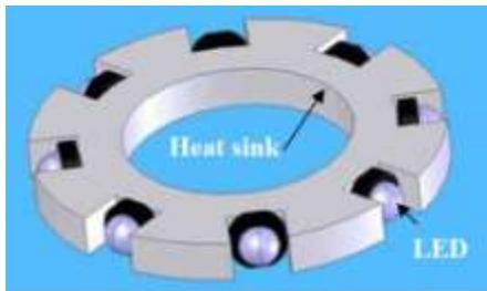
**Figure 1. Alternative LED Mounting Method**
