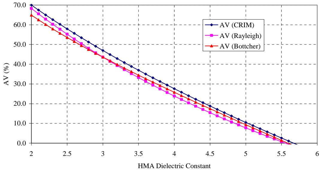
Figure 6. Air voids variations as a function of  $\epsilon_{HMA}$ .
