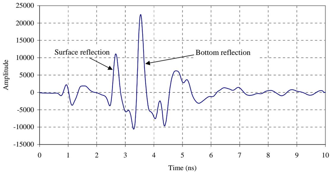
Figure 10. Typical GPR scan collected on a HMA slab.
