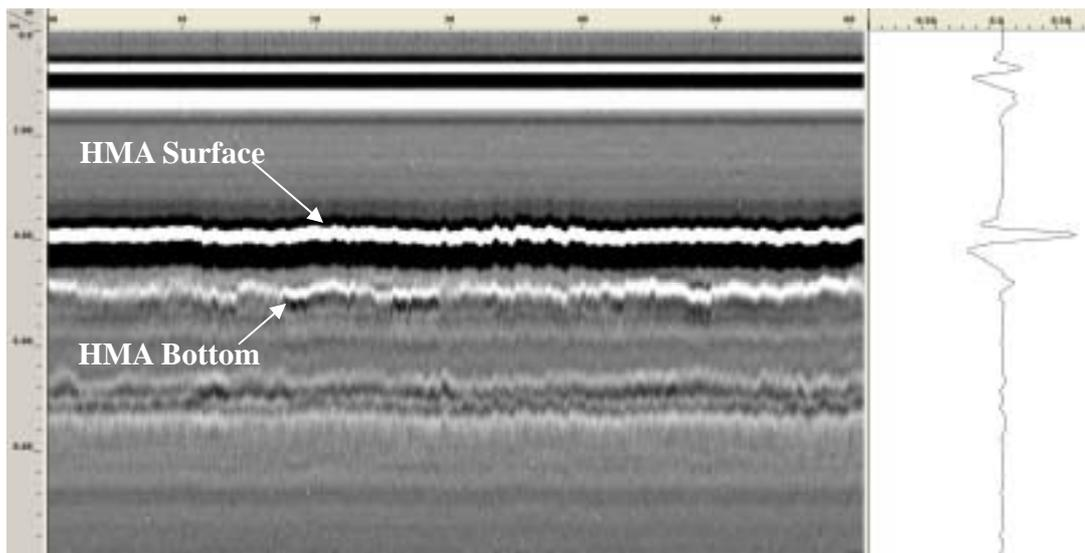
Figure 13. GPR image from the composite pavement with HMA surface.
