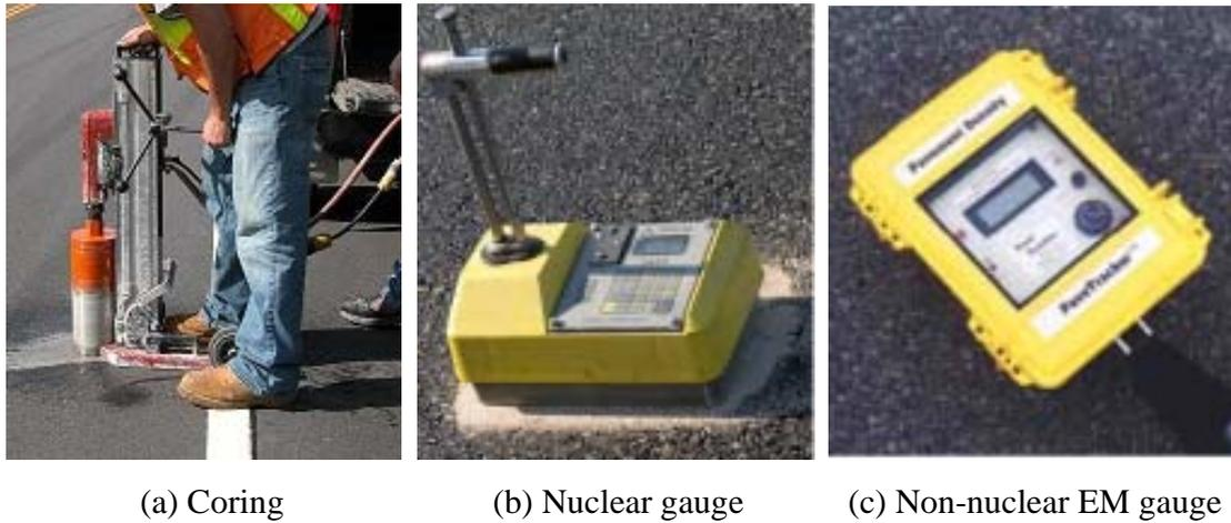
Figure 1. Available methods for density measurements for HMA airport pavements.
