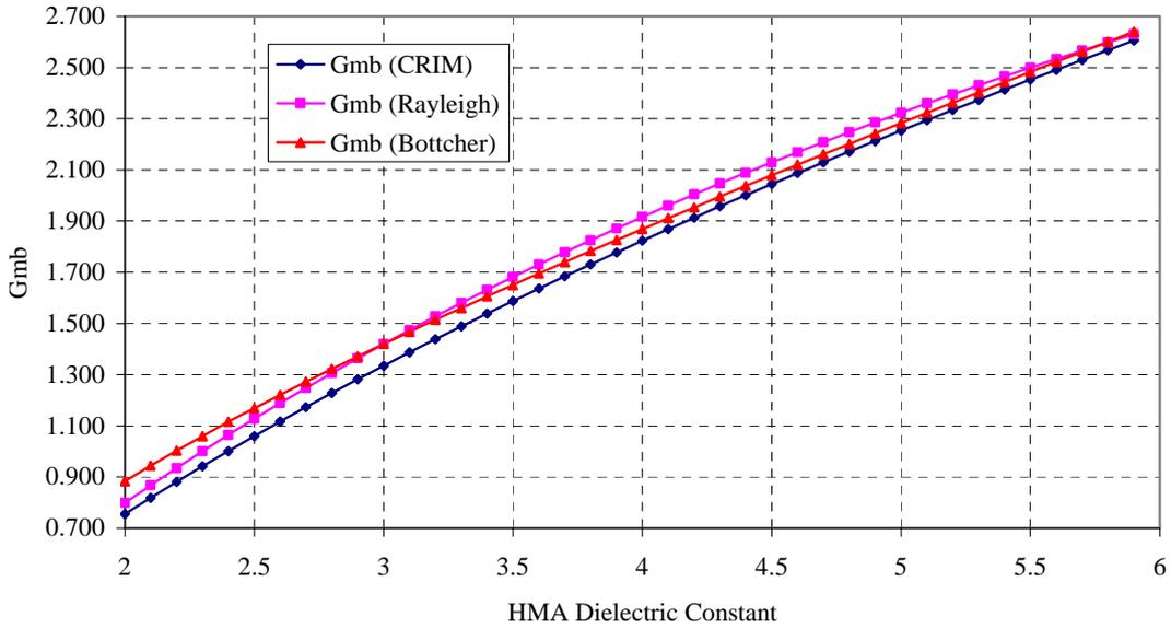
Figure 5.  $G_{mb}$  variations as a function of  $\varepsilon_{HMA}$ .
