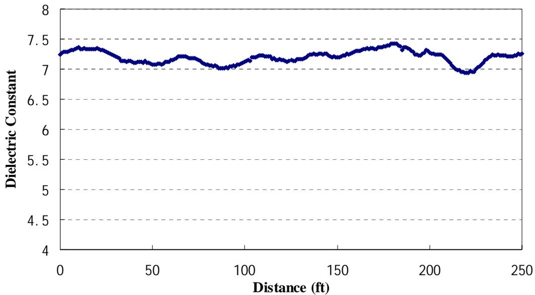
Figure 14. Dielectric constant profile of the HMA surface.
