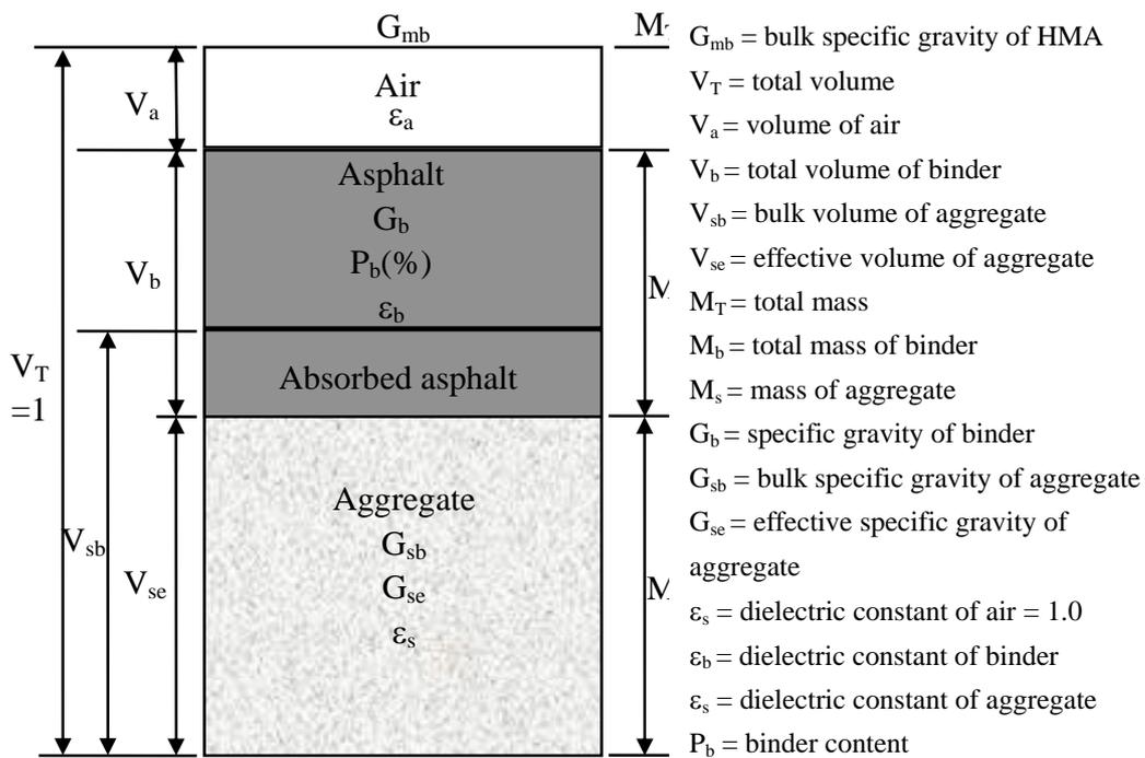
Figure 4. HMA volume and mass composition.
