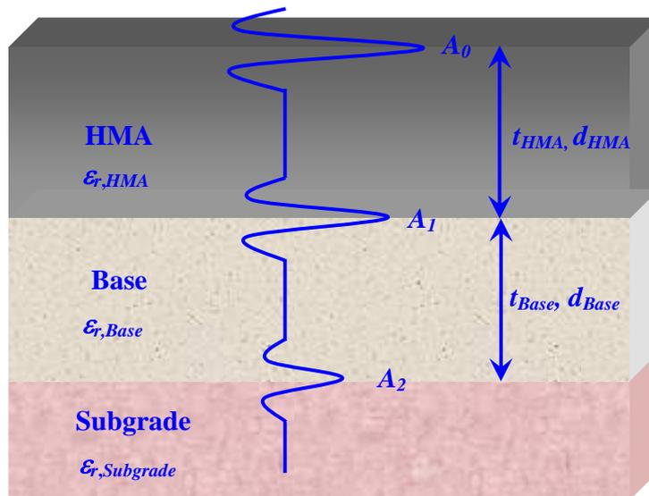
Figure 3. Typical GPR signal for an HMA pavement system.
