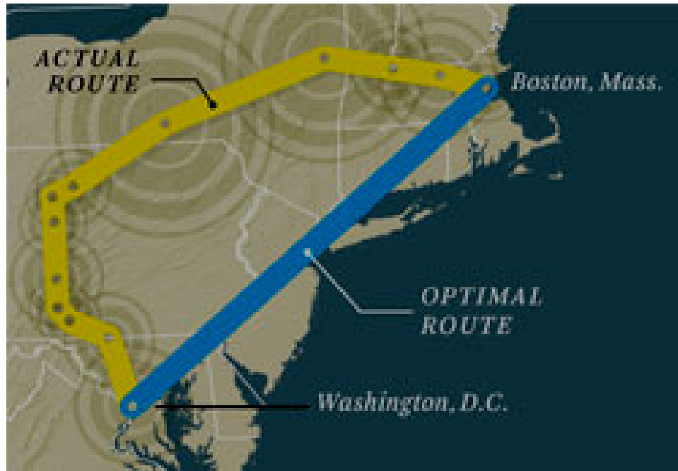
Figure 4. This 68-minute US Airways Flight 2046 (yellow) uses about 275 gal. of fuel to fly 585 miles from Washington, D.C., to Boston, Mass. The same flight under NextGen (blue) would save 23 minutes, 91 gal. and 185 miles. (Illustration by Golden Section Graphics) Peterson, B. S. (2007, August). End of Flight Delays? FAA's GPS Fix Could Bust Sky Gridlock. Retrieved February 5, 2009, from Hearst Communications, Inc.
