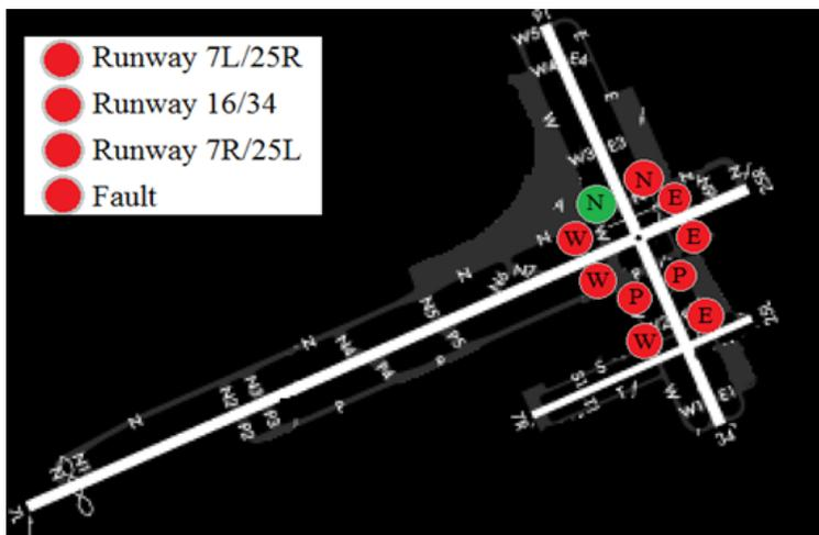
Figure 5-5. RIPLS control panel, aircraft cleared to cross 16/34 at November
