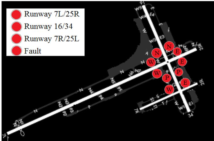
Figure 5-4. RIPLS control panel display default
